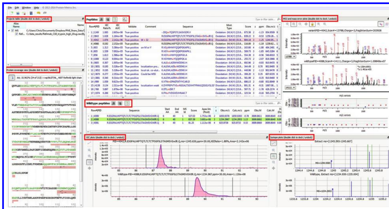
Figure 1. View of the interactive dashboard of Byologic. The red boxes highlight the different “views” of the dashboard. There is a (1) project view for the data files in use, a (2) protein (sequence) coverage view displaying the entire protein sequence along with the observed modified peptides, (3) peptides table and (4) wildtype peptides table with information such as predicted and observed masses, mass errors, XIC areas, retention times and retention time prediction, and modified-wildtype side-by-side plots in the (5) XIC plots view, (6) MS2 view showing annotations and associated fragment errors, and (7) isotope plots view for MSI data.
